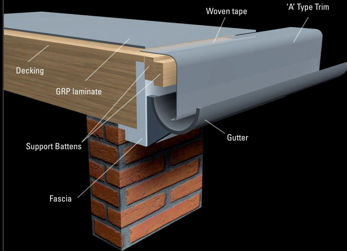
Fitted to the roof edges to allow drainage into the gutter.
