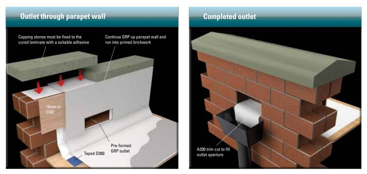
It is recommended that the pre-formed GRP outlet lining is constructed at the same time as the trims are fixed to the roof. It is possible for two D260s to be joined together using the woven glass tape in order to seal the joint after the trims have been securely fixed to the decking using clout nails.
