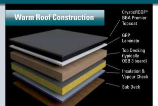
This diagram demonstrates a typical warm roof construction and can be used as a guide, however we do recommend that you check current building regulations before commencing work. Warm roof constructions generally require edge trims with a greater drop, such as the A250 and B300, due to the additional thickness of the roof.
