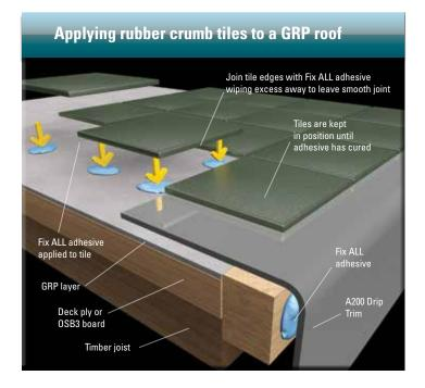
Once the GRP roof has fully cured, tiles can be applied. Preferably tiles should be laid as soon as the roof has cured with any dirt and debris being removed from the roof. If the roof has been left for any length of time and surface dirt and debris have accumulated, it will be necessary to thoroughly clean the surface. It is strongly recommended that a light sanding and surface wipe with Acetone be used to ensure the best possible adherence.
