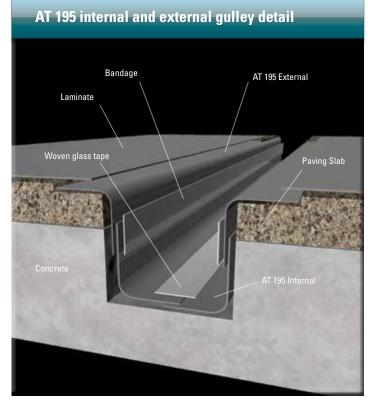
Wherever laminate is used to cover an area which runs parallel to another laminate surface, AT195 Internal and External trim is recommended.
