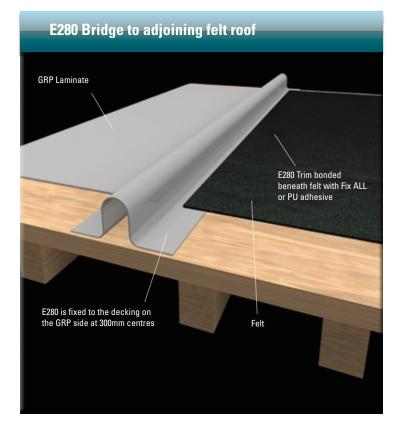
Not only is the E280 compatible with C5 closures, but it can be used for creating rolls on any ridge details, expansion joints on large roofs (50m2 or over) or to bridge GRP to felt roofs.
