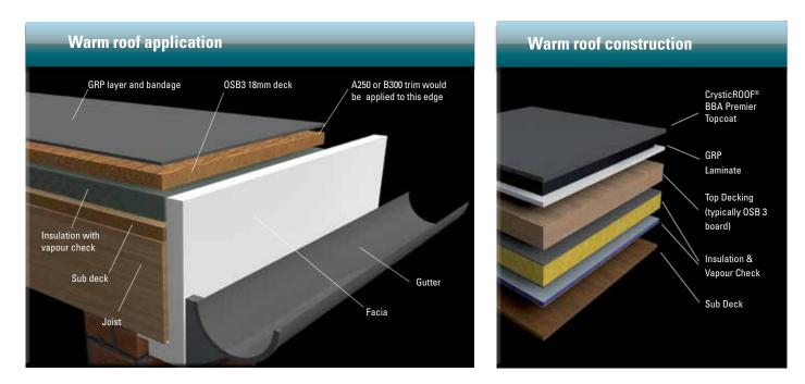
GRP roofs can be used easily to meet either a cold or a warm roof specification. When working with a warm roof, the first step will be to apply a sub-deck to the joists at 300mm centres, followed by a vapour check and laying an insulation sheet over the top. You can also buy insulation sheets with a vapour check in-situ.
