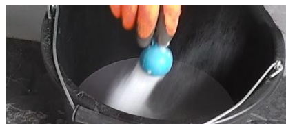
Hardener added and stirred into resin
